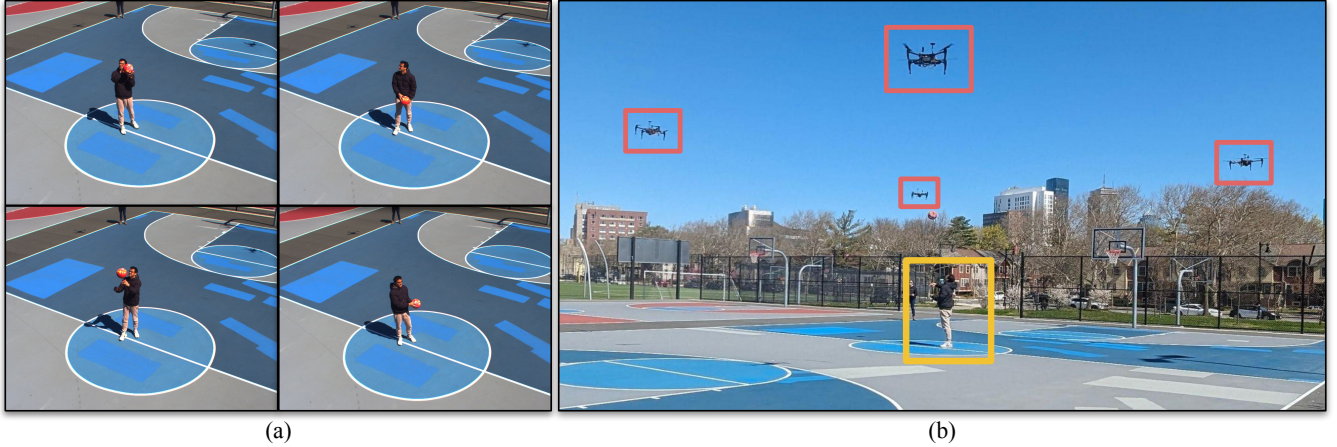
Fig. 1: We propose a novel approach to collect time-synchronized images with a fleet of UAVs for mapping dynamic scenes in unstructured outdoor environments. In our system, we utilize GNSS-PPS to synchronize cameras across UAVs and collect two dataset sequences to generate 4D maps of dynamic scenes. (a) shows the data from one out of four UAVs spanning multiple timesteps and (b) shows the multi-view data collection system at a single timestep from the sequence.
